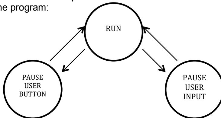
From the *Run* state we can move to the *PauseUserButton* state if the button is pressed. From the *Run* state we can move to the *PauseUserInput* state if the user types a 'p'. We can only exit the *PauseUserButton* to the *Run* state if the user releases the button. Likewise, we can only exit the *PauseUserInput* state if the user types a character 'r'. Note that all the state machine is wrapped around a `while(1)` and implemented as a `switch` statement.
